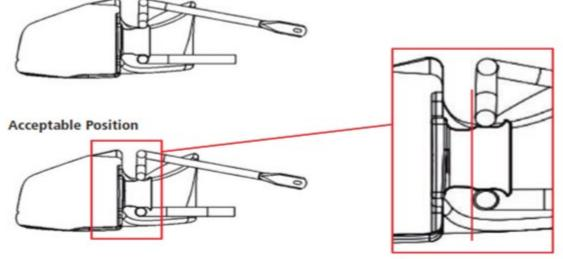
Not acceptable position If any part of the tubes of the front bumper are in the areas marked "A".
